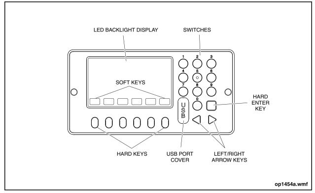
Figure 19: Operator's Display Keyboard (ODK)
