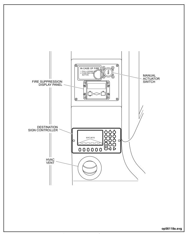
Figure 13: Driver's Overhead Panel
