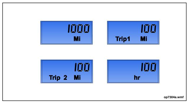
Figure 24: Odometer/Hourmeter Display Screen Options
