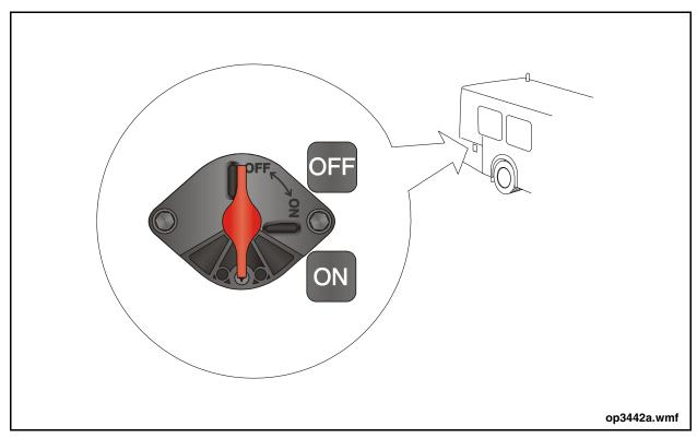
Figure 1: Battery Disconnect Switch
