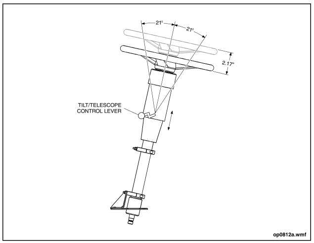
Figure 16: Steering Wheel Adjustment
