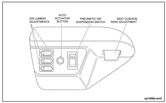
Figure 15: Driver's Seat Switch Panel
