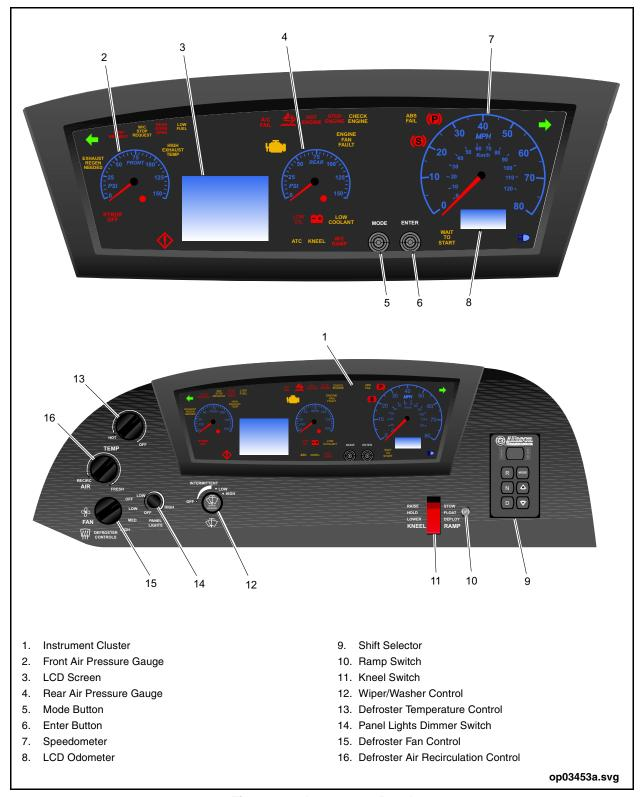
Figure 22: Instrument Panel
