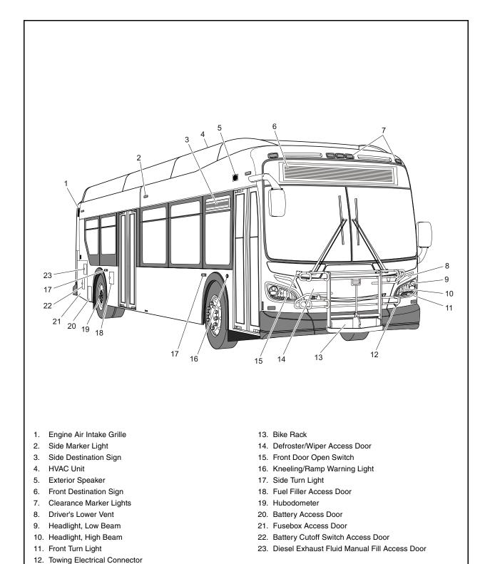
Figure 9: Front Exterior View
