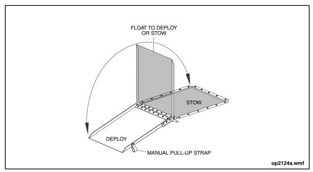
Figure 35: Wheelchair Ramp Operation
