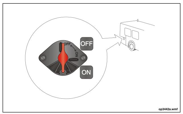
Figure 32: Battery Disconnect Switch
