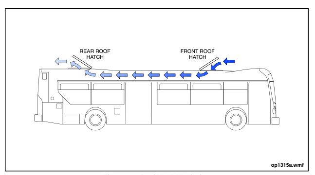
Figure 34: Roof Hatch Ventilation
