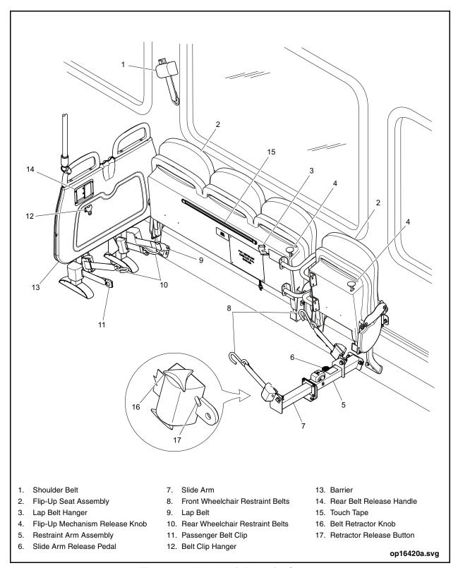
Figure 36: Wheelchair Restraint System
