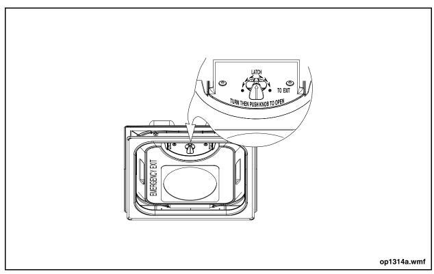
Figure 3: Roof Hatch Emergency Exit
